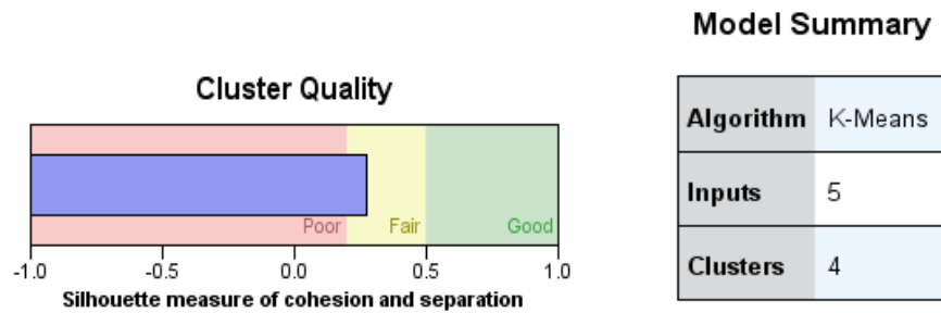
Figure 4. Running k-means algorithm, cluster quality and model summary
